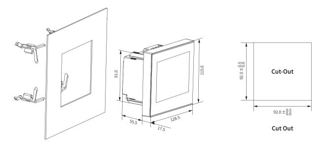
**I/O Module Dimensions** Unit: mm
